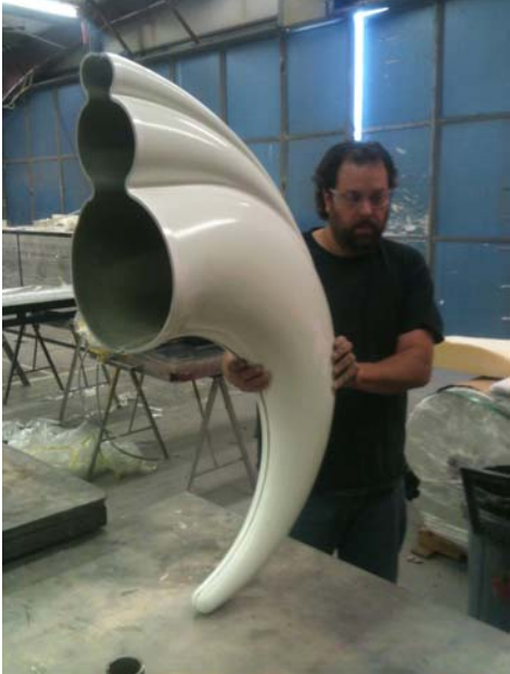
3D Rhino Model for STL, Fiberglass Negative Mold, Fiberglass Positives
